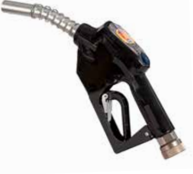
Art. 093-5210-000 Automatic nozzle "PA60" for diesel fuel transfer Flow rate 70 l/min Aluminium body Swivel connection F 1"
