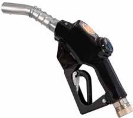
Art. 093-5220-000 Automatic nozzle "PA120" for diesel fuel transfer Flow rate 120 l/min Aluminium body Swivel connection F 1"
